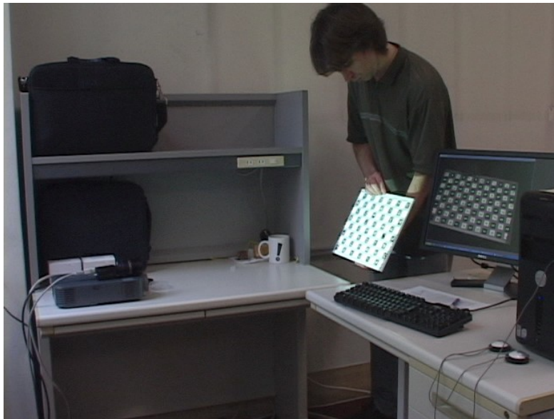
Figure 1.2: Snapshot of our demo video showing the test user calibrating a casually installed projector-camera system.
