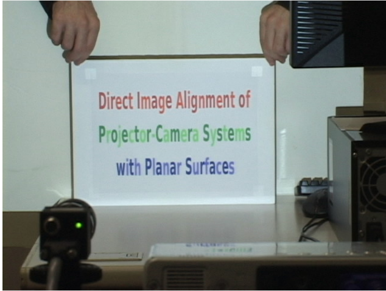
Figure 1.1: Snapshot of our demo video showing the patterns of Figure 5.5, where the system has aligned the projector displayed pattern with the printed one.
