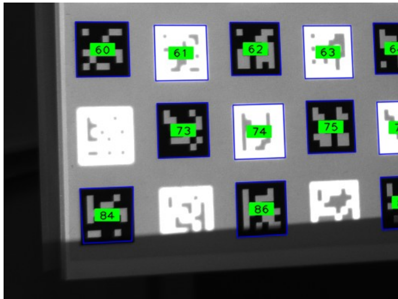
Figure 3.7: Lower left area of the detected markers from Figure 3.5. We can observe severe defocusing of projector markers.
